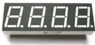
Image 1 shows a four digit seven-segment indicator. Each category has seven LEDs which illuminate the appropriate segments. Unlike graphic displays indicators are cheaper to manufacture and they reduce the cost of a device.
