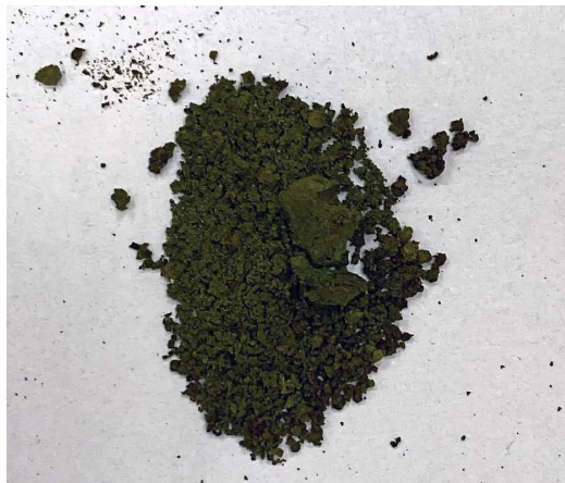
Fig. 3. General view of the melt after the alkaline leaching process
