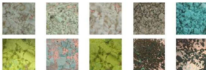
Fig. 1. The dried dispersions of positively charged particles based on zinc ferrocyanides (top) and ferricyanides (down) with chemisorbed cations with an electron-deficient incomplete coordination sphere (from left to right: K^+ , La^{3+} , Zn^{2+} , Cu^{2+} , Co^{2+} ).
