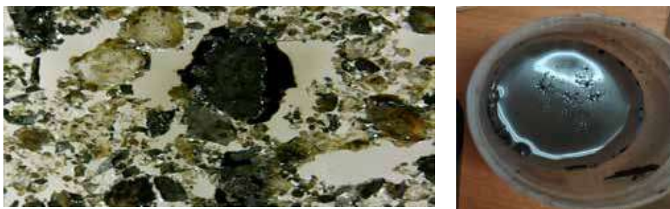
Fig. 4. Investigation of contaminated soil: a – microscopy of the surface layer of the water extract of contaminated soil. Sample № 1; b – a bowl with a mixture of soil sample № 1 and distilled water
