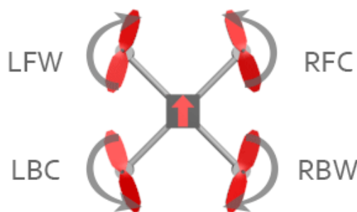
Fig.1 Direction of rotation of the screws and location of the motors.
