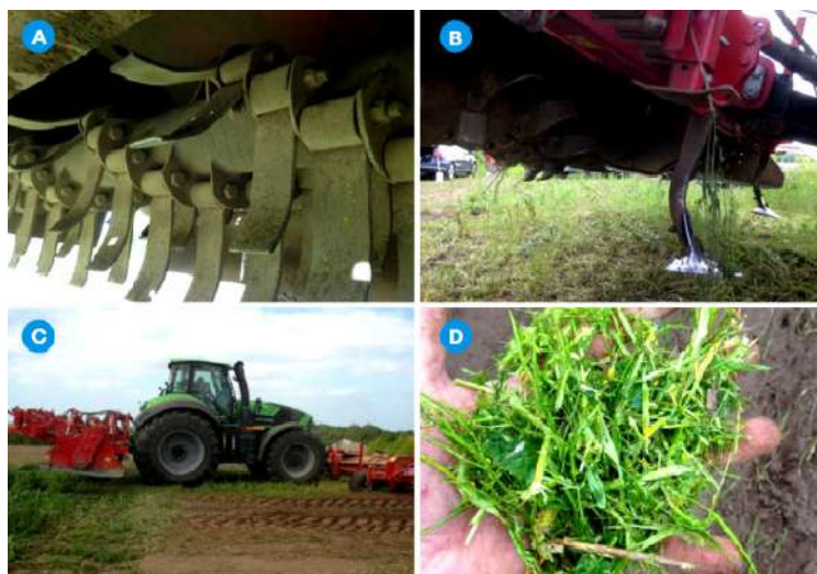
Figure 2.8.1 – Single-pass biofumigation system: A = tine arrangement on a haulm topper, B = rotavator with rigid tines and S-blades, C = a single-pass system using front-mounted haulm topper and rear-mounted rotavator, and D = good-quality brassica residues following maceration (AHDB PCN, 2020)
